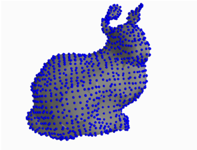
Fig. 3. The bunny reconstructed by SCD embedding. The approximate geometry of the bunny has been recovered, although the bunny appears inflated and somewhat distorted. The embedding recovers only the positions of the nodes, the triangulated surface mesh is
